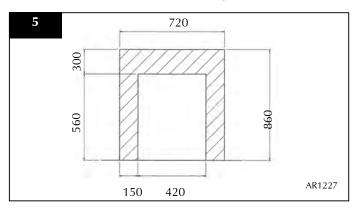
4.5 The maximum depth of combustible shelf is 150mm at a minimum height of 300mm above the fireplace opening.
